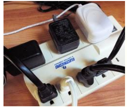
Small household "wall warts" are typically noisy switching power supplies.
