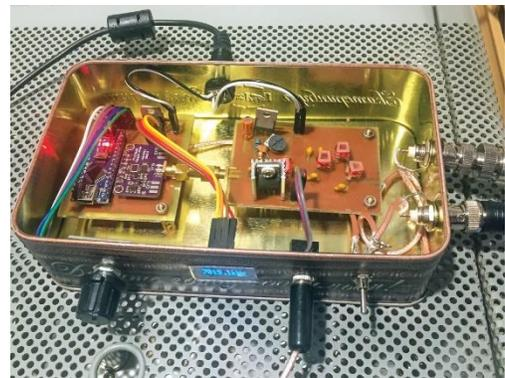
Here, we take another step forward. The Tuna Tin "S" (for synthesized) keeps costs below \$20 and is still small enough to fit within the confines of a tuna tin, but has an integral VFO, digital display, and a higher power MOSFET final.
