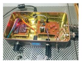
Here, we take another step forward. The Tuna Tin "S" (for synthesized) keeps costs below \$20 and is still small enough to fit within the confines of a tuna tin, but has an integral VFO, digital display, and a higher power MOSFET final.
