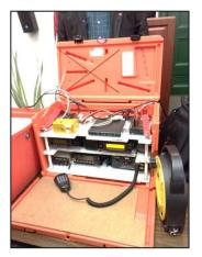
I had previously built an all-thread go box but how nice to meet Norm for his ideas! He used all-thread with small pvc pipe holding each shelf up. There's also a cloth red strap so he can lift the shelf system out of the box. Noticed he notched the shelves for cords? Small details are priceless if we share them.
