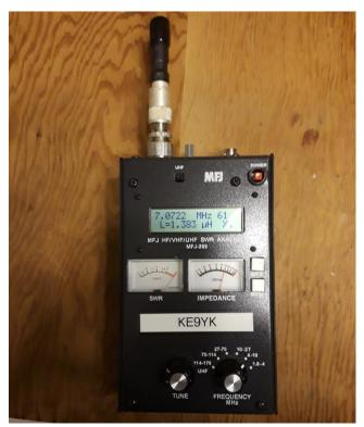
On to build the high frequency coil, but ready to use checking antenna traps.
