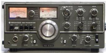
Notice there are no MENU buttons. All switches, knobs and dials are plainly labeled as to their single function. One did have to learn how to properly tune the transmitter with the three Load, Plate and Drive controls but that was easy to master. Tubes were used in the final amplifier and they were very forgiving as you learned the ropes. If you did have any questions, the club Elmers were great about teaching you the ropes.
